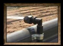
OPTIONAL SPRINKLER SYSTEM-Priefert's sprinkler system enhances the drag's effectiveness and keeps the ground moist to eliminate dust. Just attach any outdoor water hose to the walker's sprinkler hookup and you are ready to go. This add-on is a great addition to any Panel Walker system.
