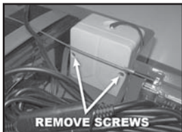
Fig 16 - Circuit Board Box
